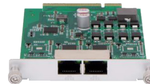
Dual Gigabit Ethernet ports
