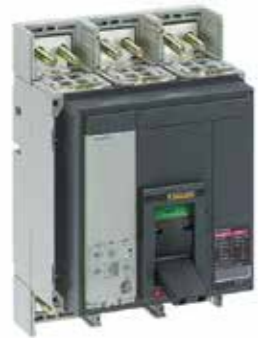
NS16N3F20X ComPact NS 1600, H type (Icu = Ics = 50kA), 3 poles, Fixed type, Micrologic 2.0, No charging motor, front connections
