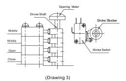
Adjustment of Middle Position Switch (Drawing 3)
