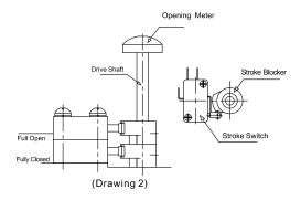
Adjustment of Limit Position Switch(Drawing2)
