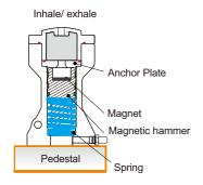
(2) The hammer instantly drops down when air pressure overcomes the strength of Magnet to cause a downward impact.
