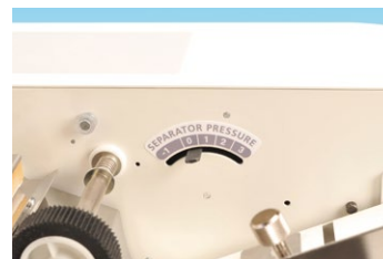
Separator pressure adjustment prevents double feeds.
