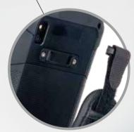
Quick-release hand strap saves time in battery replacement
