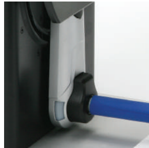
Colored LED indicator provides rewinder operation status
