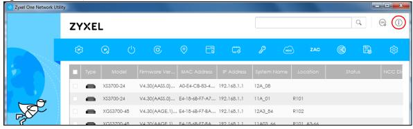
3 Select a network adapter to which your supported devices are connected.
