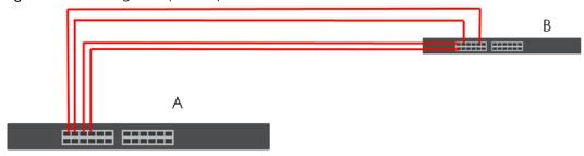
2 Configure static trunking - Click Advanced Application > Link Aggregation > Link Aggregation Setting. In this screen activate trunk group T1, select the traffic distribution algorithm used by this group and select the ports that should belong to this group as shown in the figure below. Click Apply when you are done.
