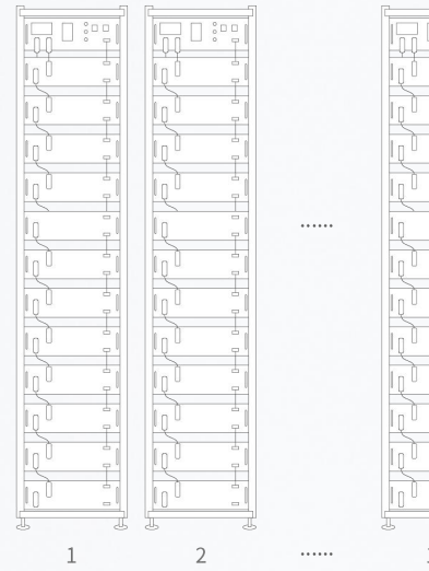
Maximum support for 10 inverters in AC parallel operation
