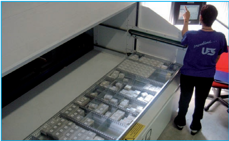
Automatic load system for final products
