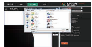
整理測量完畢刀具之刀長並輸出 CNC 刀長補正式碼 Sort out the tool length of the tool after measurement and output the CNC tool length compensate code
