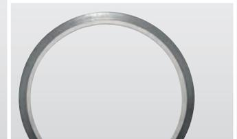
**Style CG** – Is comprised of a sealing element and outer metal ring. The outer ring assists in locating the gasket on the mating flange faces and prevents over compression of the sealing element ensuring optimum sealing performance. Style CG gaskets are suitable for use on raised and flat faced flanged connections. Style CG gaskets are suitable for use in mild to moderate service conditions.
