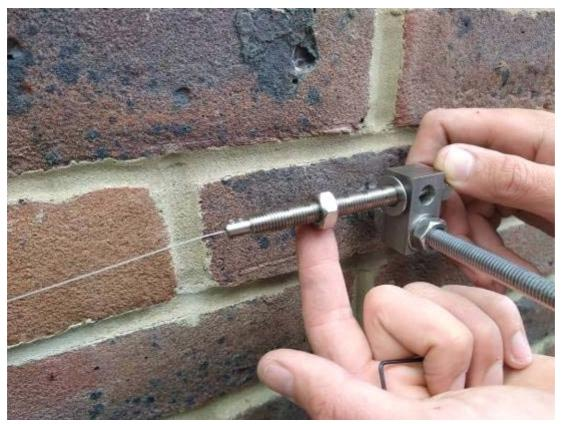
Using the graduated scale and the face of the wire clamp adjust the transducer to its preferred staring position.
