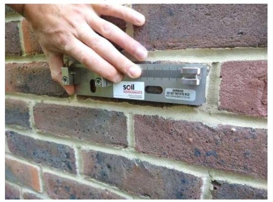
Mark the fixing hole positions using the marker pen
