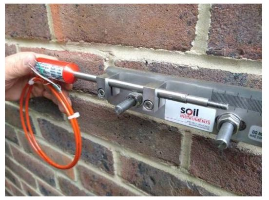
Slide the anti-rotation block over the shaft of the transducer up to the end of the body tube.
