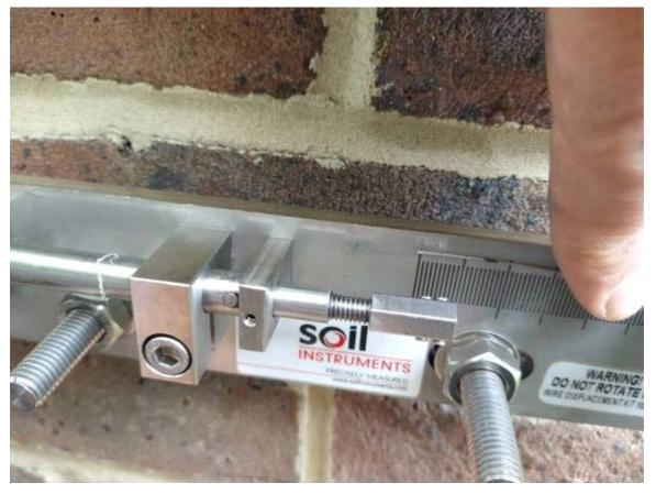
Loosen the socket set screws in the wire clamp and insert the wire, the mark should be level with the end of the clamp.
