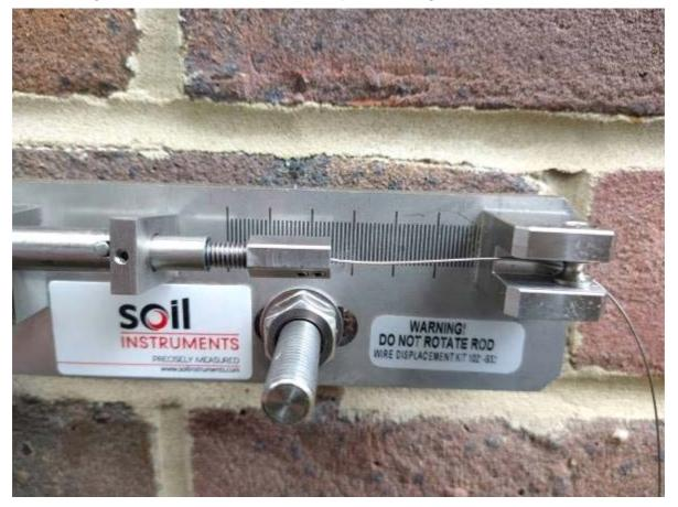
The positioning prevents the transducer being over extended should the wire be accidentally pulled beyond the range or the transducer.
