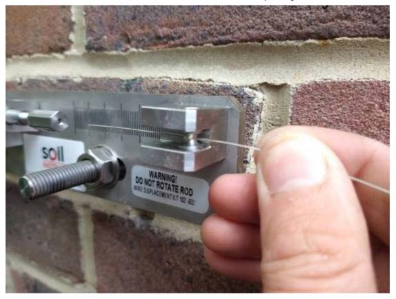
Using the graduated scale apply a mark approximately 15mm from the end of the wire.
