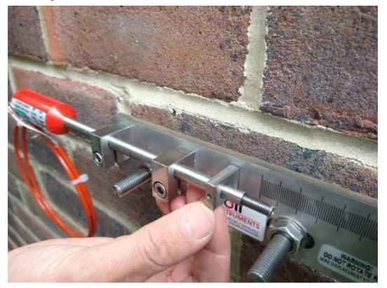
Attach the transducer wire clamp to the end of the transducer shaft and tighten using the adjustable spanner, do not over tighten.
