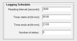
'Number of retries' enables you to set the number of times VWlog2 will attempt to re-take the reading if the reading frequency is beyond the range between Hz\_min and Hz-max. You can set the number of retries between 0 and 5.
