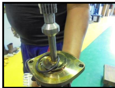
Fig 20. Cleaning Gear Torque Switch
