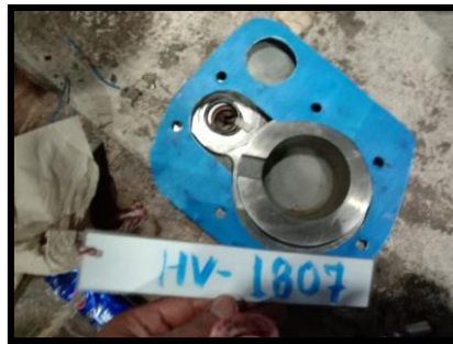
Fig 32. Change New O-ring
