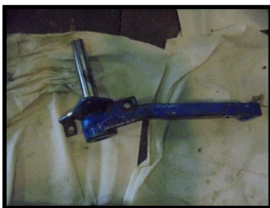
Fig 23. Cleaning Declutch Lever
