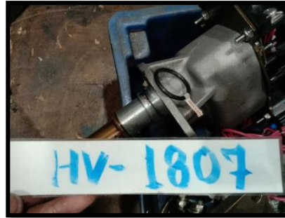
Fig 30. Change New O-ring
