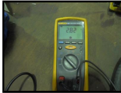
Fig 43. Coil Resistance 2 Test
