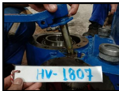
Fig 22. Cleaning Shaft Hand Wheel
