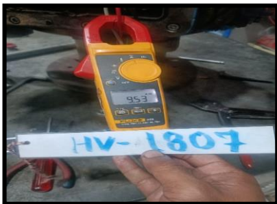
Fig 48. Current of Phase 1 Test (After)
