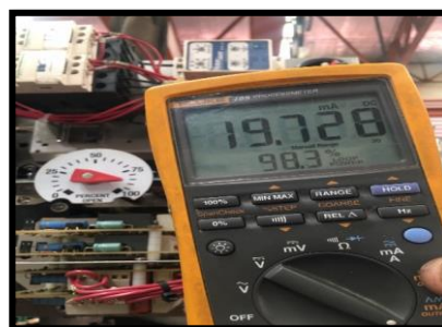
Fig 6. Feedback Signal 100% (Before)
