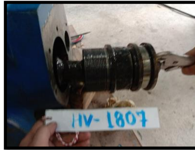
Fig 10. Inspect Spring Torque
