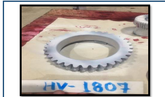
Fig 26. Inspection by Penetrant Testing ( PT Test ) Worm Gear
