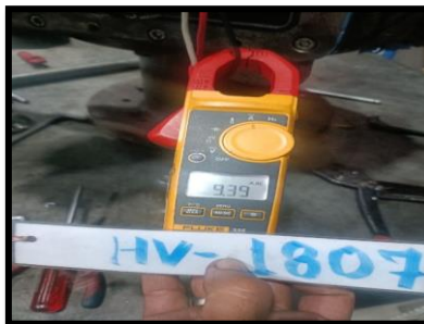
Fig 49. Current of Phase 2 Test (After)
