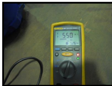
Fig 45. Insulation U1-G Test
