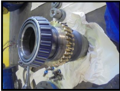
Fig 17. Cleaning Center Column
