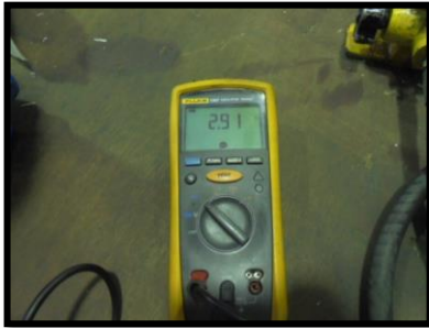
Fig 42. Coil Resistance 1 Test
