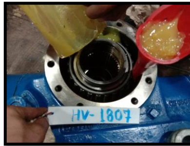
Fig 38. Change New Grease
