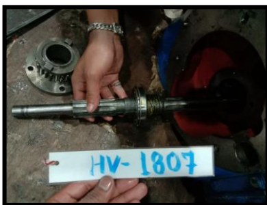
Fig 21. Cleaning Gear Shaft Motor
