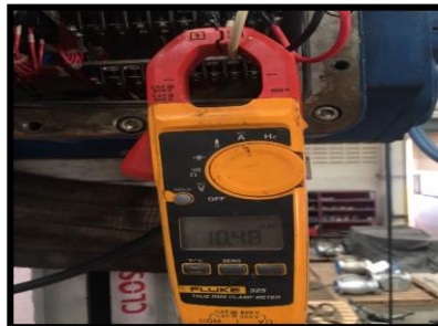
Fig 2. Current of Phase 1 (Before)
