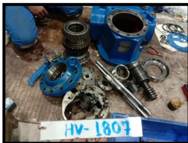
Fig 7. Remove Actuator at Shop
