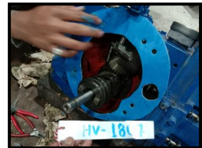
Fig 36. Change New Gasket
