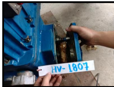
Fig 14. Inspect Shaft Hand Wheel
