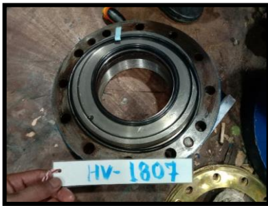
Fig 33. Change New O-ring
