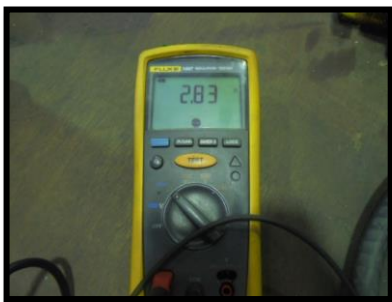
Fig 44. Coil Resistance 3 Test
