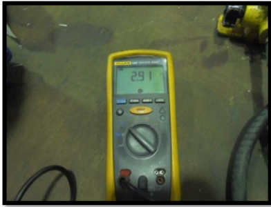
Fig 42. Coil Resistance 1 Test
