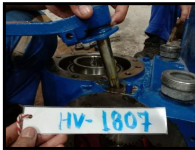
Fig 22. Cleaning Shaft Hand Wheel
