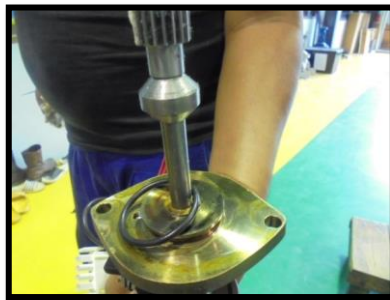
Fig 20. Cleaning Gear Torque Switch
