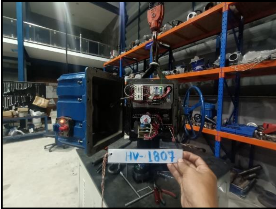
Fig 51. Disassembly Gear Torque Switch
