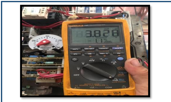
Fig 5. Feedback Signal 0% (Before)
