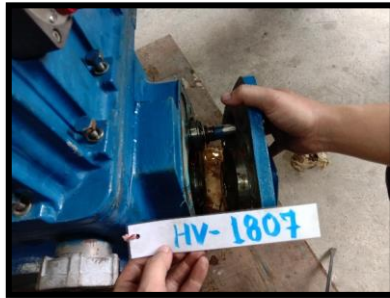
Fig 14. Inspect Shaft Hand Wheel
