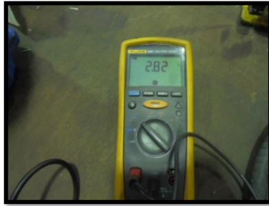
Fig 43. Coil Resistance 2 Test
