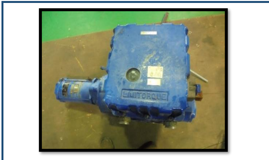
Fig 1. Visual Check the Actuator at Shop
