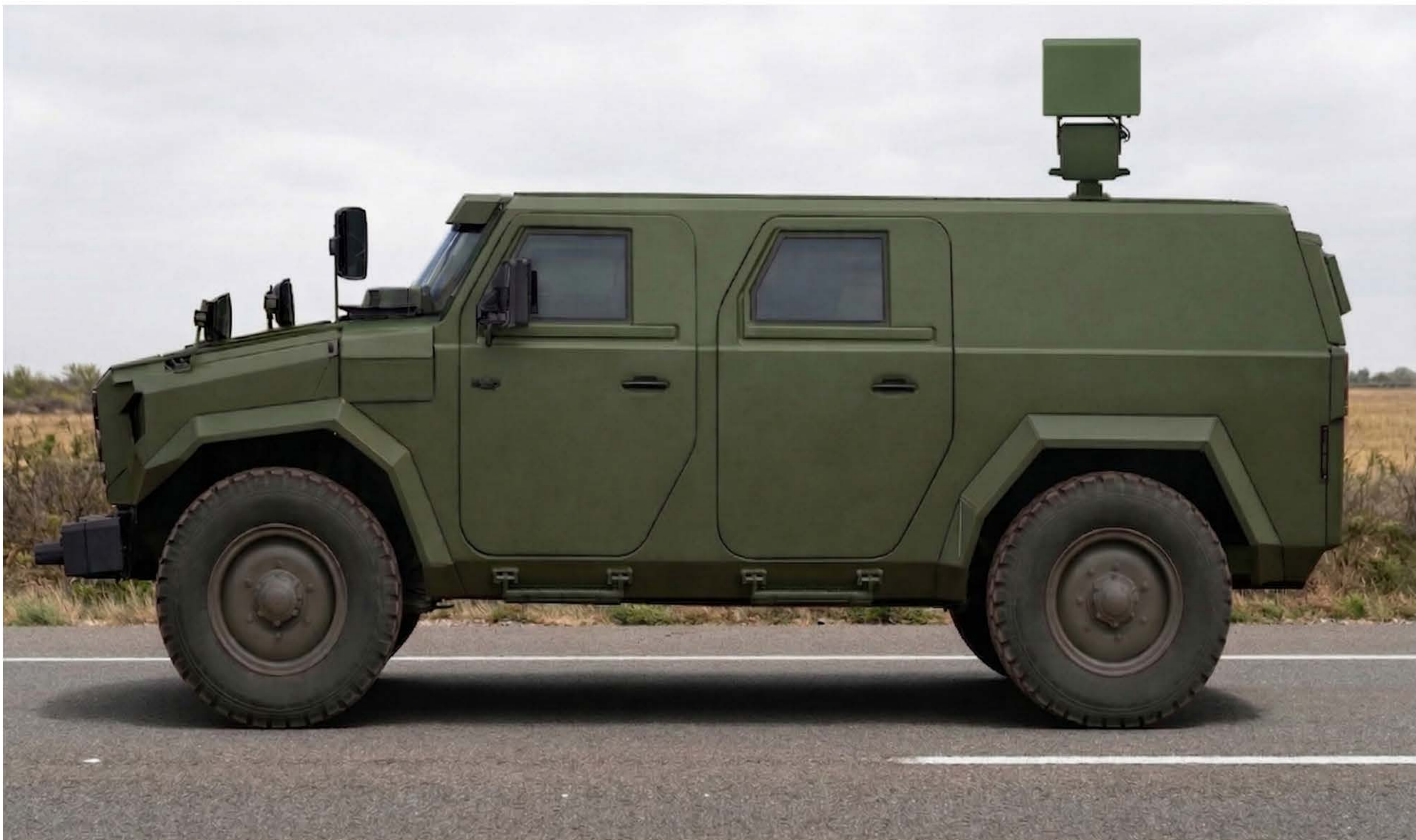
Figure: Directional Jammer JP-10C mounted on Anti-Drone Vehicle
