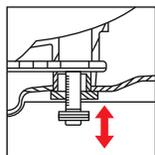
Clean up the floating valve : Pull up the floating valve can be drop and clean. Then installed back to the properly position.
