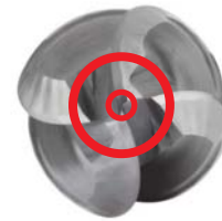
At the tip of the tool, only the center cutting edges exist. The rotational velocity is zero in the center.
