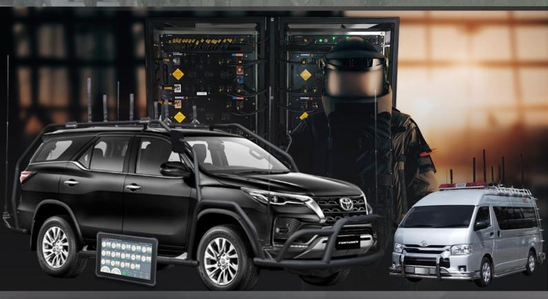
Multiband jammer DMJ-1200 is device designed for EOD mission. It broadcasts one or many jamming signals covering remote control, radio and cellular frequency band to prevent radio activated bomb.
