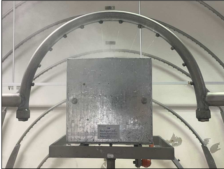
Photo No.5 : IPX4 Water test
