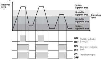
• In Dark ON mode, the waveforms are reversed.
