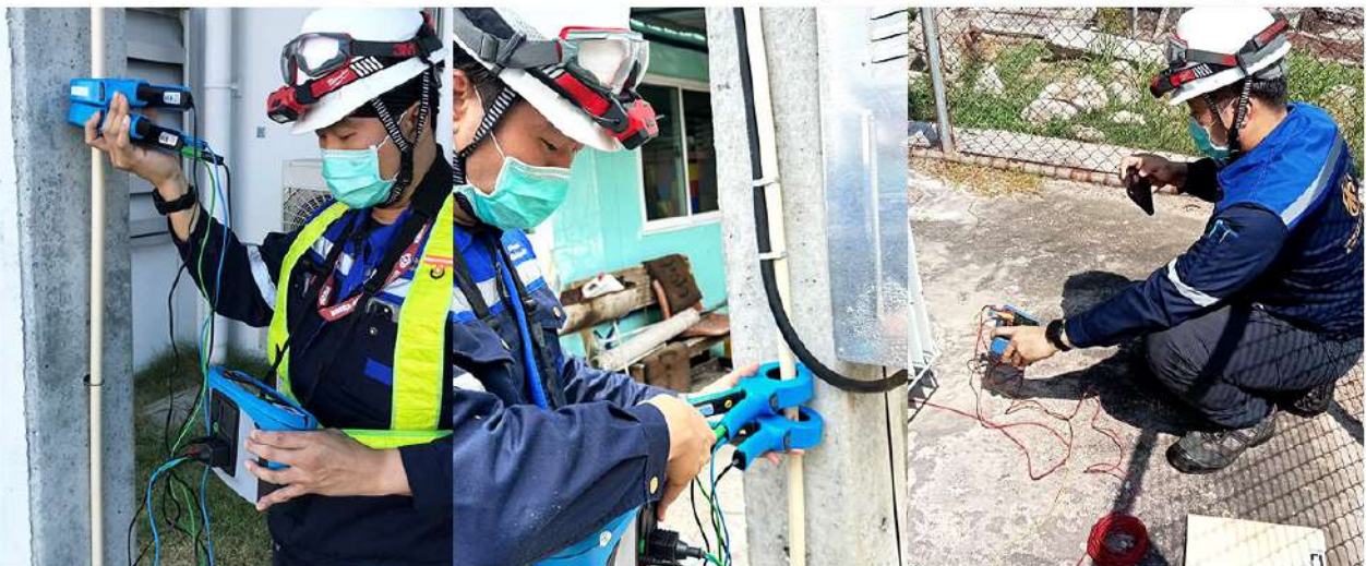
Figure 5.7: Contactless earthing resistance measurement
