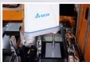
Touch Screen Inspection
