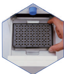
Step2 Put the adapter plate
