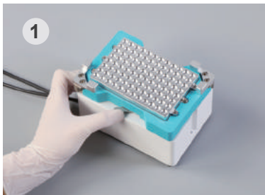
1 Toggle the handle on the back of the instrument
