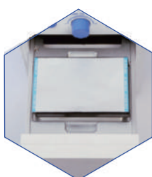
Step3-1 Put a sealing film
