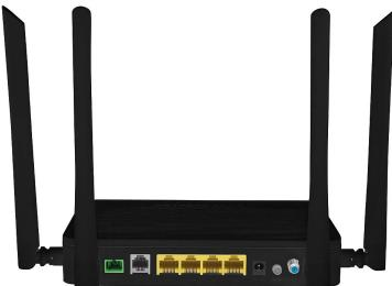
1. The ONTG-4G1FTW-H optical receiver enables data (internet) distribution through fibre optic infrastructure (Passive Optical Network). It is equipped with a FXS (POTS) port to be able to connect analog telephone devices, 4 GE ports and a CATV RF output.
