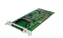
**GX-4C2CI-BP-00** receiver module is equipped with one RF coaxial input connector (F Female) and two PCMCIA Common Interface slots. The module is able to tune up to **four DVB-C digital QAM multiplexes,** decrypt the scrambled programs through the C.I. slots and share and pool the contents to the **GALAXIA** main chassis.
