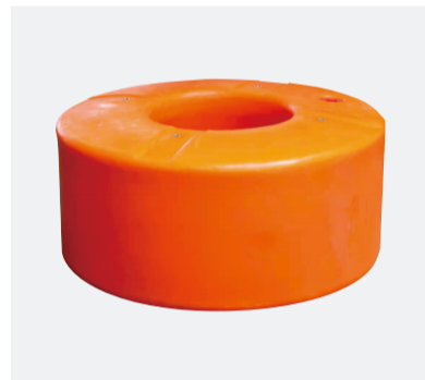
Floating ring (round): 800X350X350mm weight 12.5 kg, buoyancy 120 kg
