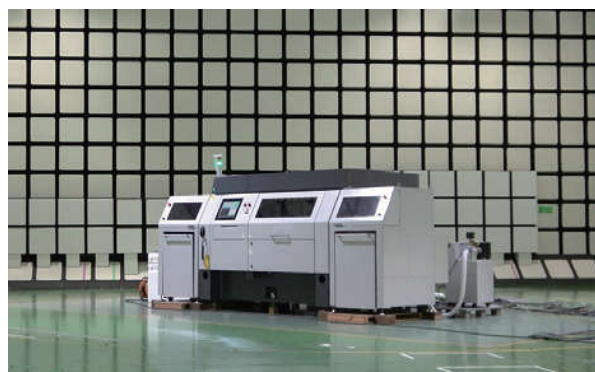
One of the largest radio-frequency anechoic chambers in Japan
