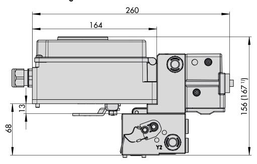
1) For attachment using intermediate plate
