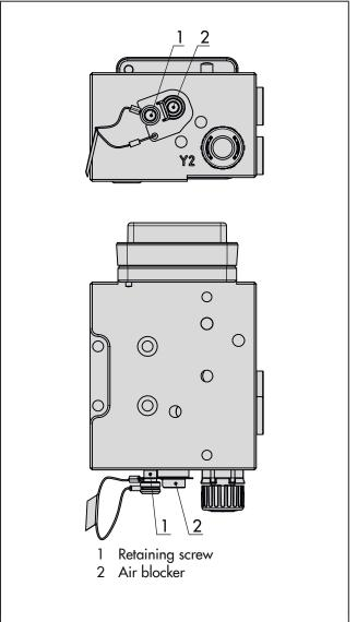
Fig. 5-15: Adapter block for attachment according to VDI/VDE 3847-2
