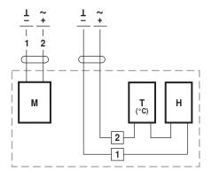
M = Actuator T (°C) = Thermostat H = Heating
