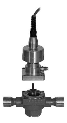
4. Install the new bolts supplied with the adaptor. Tighten in a star cross pattern to 10-foot pounds of torque.
