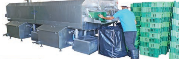
DUAL-LANE WITH 4 WASHING ZONE + BLOW OFF
