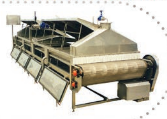
• STEAM TUNNEL COOKER
