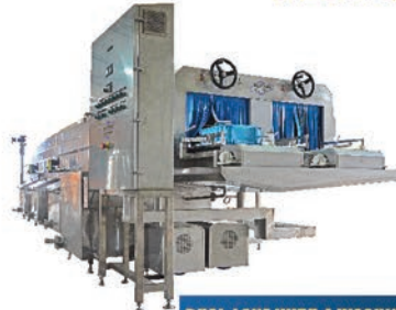
DUAL-LANE WITH 4 WASHING ZONE + BLOW OFF
