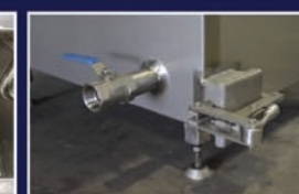
DRAIN DOOR & DRAIN VALVE
