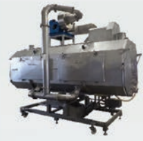
Drum Dryer (Heater)
