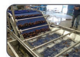
• FLUME WASHER CONVEYOR
