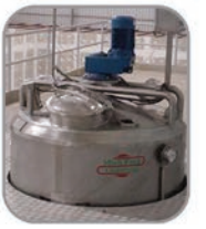
• MIXING TANK (HANGING)
