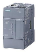
SIMATIC S7-1200 G2: compact CPU 1212C DC/DC/RLY; power supply: DC 20.4-28.8 V DC; onboard I/O: 8x DI 24 V DC; 6 DO relay 2 A; memory: program 150 KB data: 500 KB, retentivity: 20 KB
