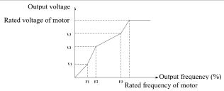
Fig. 7-19 Schematic Diagram of Multi-point Polyline V/F Curve
