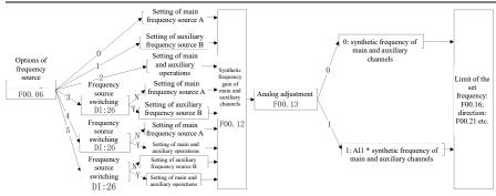
Fig. 1-1 Schematic Diagram of Speed Input Mode
