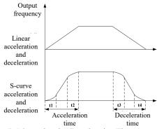
Fig. 7-16 Acceleration/Deceleration Time Control Diagram
