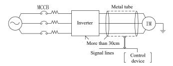
Fig. 3-8 Solution to Inductive Interference
