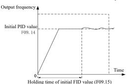
Fig. 9-29 Schematic Diagram of Initial PID Output
