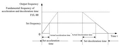
Fig. 7-33 Schematic Diagram of Acceleration and Deceleration Time
