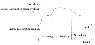
Fig. 7-39 Schematic Diagram of Energy Consumption Braking
