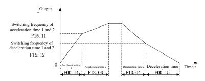
Fig. 7-34 Schematic Diagram of Automatic Switching of Acceleration and Deceleration
