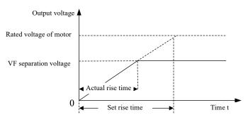
Fig. 7-20 Rise Time Description of VF Separation Voltage
