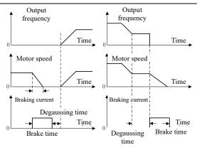
Fig. 7-17 DC Braking Process for Start Fig. 7-18 DC Braking Process for Stop
