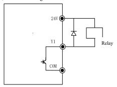
Fig. 3-15 Wiring of Multi-function Output Terminals
