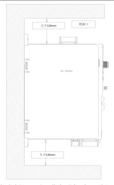
Fig. 2-2 Inverter Installation Direction and Space
