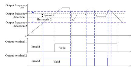
Fig. 7-37 Schematic Diagram of FDT Detection
