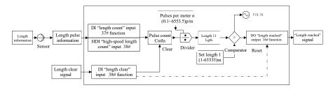
Figure 7-40 Block Diagram of Fixed-length Counting
