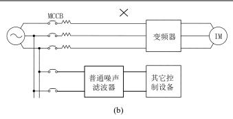
Fig. 3-6 Incorrect Installation of Noise Filter
