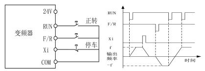
(a) Wiring diagram of three-line control (F00.03=2) (b) Forward/reverse running logic (F04.19=0, F00.03=2)
