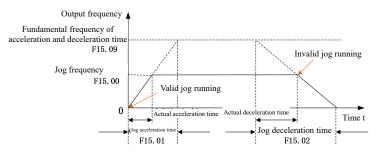
Fig. 7-32 Schematic Diagram of Jog Running
