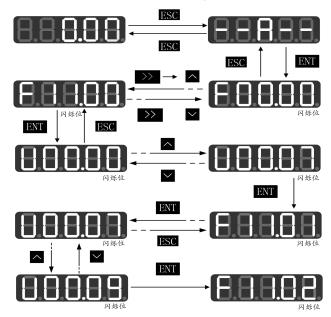
Fig. 4-4 Example of User-defined Mode Setting
