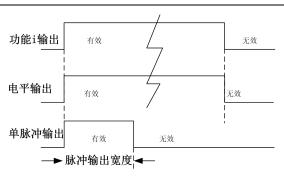
Fig. 7-13 Schematic Diagram of Level and Single Pulse Output of Digital Output Terminal The digital output terminal Y1 and relay output terminal R1 have two output types: level and single pulse, as shown in Fig. 7-13. For the level output, the output status of the function terminal is consistent with the function status; and for the single pulse output, the active level of a certain pulse width will not be outputted until the function is enabled.
