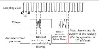
Fig. 7-13 Schematic Diagram of Terminal Filter Sampling
