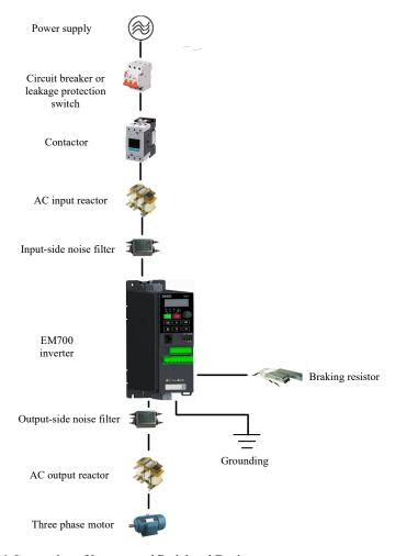
Fig. 3-1 Connection of Inverter and Peripheral Devices
