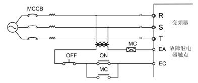
Fig. 3-4 Connection of Input Circuit Breaker
