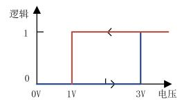
Fig. 7-10 Correspondence between Analog Input Terminal Voltage and Current Logic
