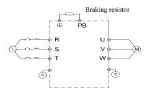
Fig. 3-3 Standard Wiring of Main Circuit
