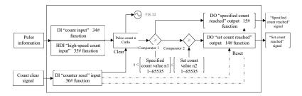
Fig. 7-42 Block Diagram of Counting Function
