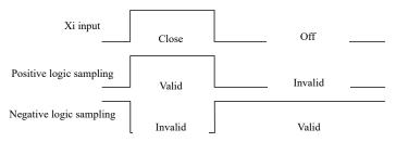
Fig. 7-12 Schematic Diagram of Positive/Negative Logic Sampling of Terminal When the bit is set to 0, the multi-function input terminal is valid in the closed status and invalid in the open status;
