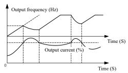
Fig. 7-25 Current Limit Process
