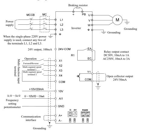
Fig. 3-19 Standard Wiring Diagram of Control Circuit
