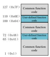
Fig. 12-21 Classification of MODBUS Function Codes
