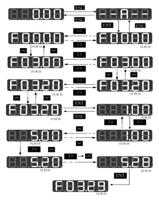
Fig. 4-3 Flowchart from Power-on to F03.28=5.28 Setting
