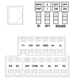
Fig. 3-11 Layout of Control Circuit Terminals
