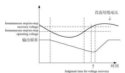
Fig. 7-24 Schematic Diagram of Instantaneous Stop/Non-stop Deceleration Function
