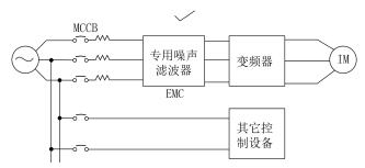
Fig. 3-5 Correct Installation of Noise Filter
