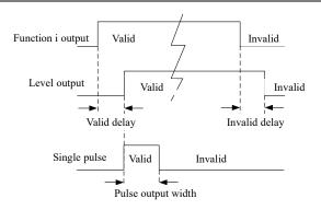
Fig. 7-15 Schematic Diagram of Level and Single Pulse Output of Digital Output Terminal
