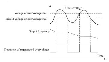
Fig. 7-23 Schematic Diagram of Overvoltage Stall Protection
