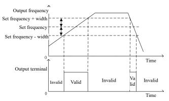
Fig. 7-36 Schematic Diagram of FAR Detection
