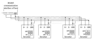
Fig. 3-17 Wiring of Communication Terminals of Multiple Inverters
