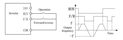
(a) Wiring diagram of two-line control (F00.03=0) (b) Forward/reverse running logic (F04.19=0, F00.03=0)
