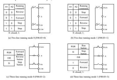
Fig. 1-6 Control Logic Diagram of Terminal Operation
