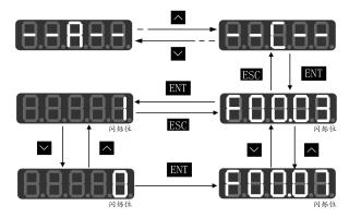
Fig. 4-5 Function Code Modification in Non-default Mode
