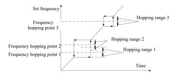
Fig. 7-35 Schematic Diagram of Frequency Hopping
