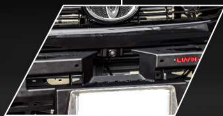
COVER PLATE Can be opened for Sonar Box and Camera
